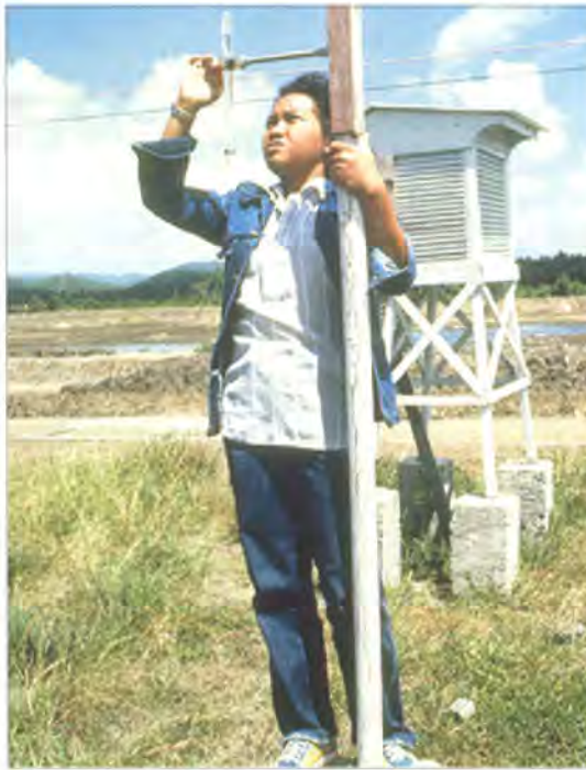
Volunteer measuring the rate of evaporation of water using a Piche evaporimeter; behind is a traditional "Stevenson screen" instrument housing
