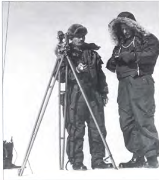
During the International Geophysical Year, an increased programme of weather observations in the higher atmosphere was implemented world-wide; shown is a sun observation on an ice shelf in Antarctica for precise positioning (US Navy)
