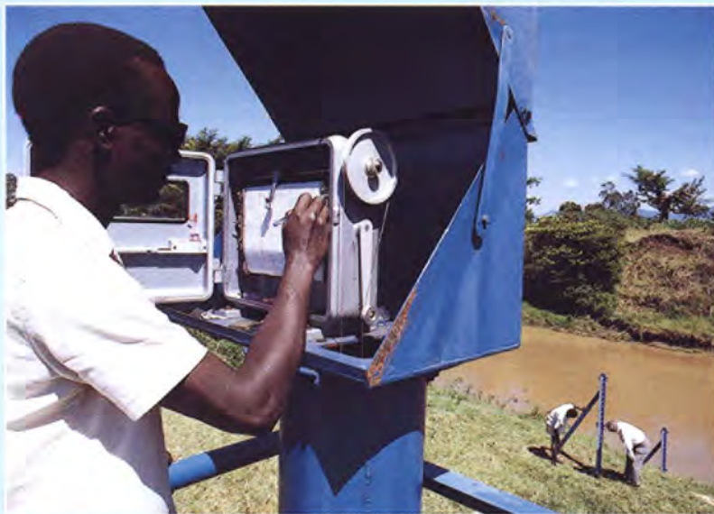
A volunteer (right) learns to use a staff gauge; his readings can be compared with those from the automatic water level recorder in the foreground (P. Mosley)
